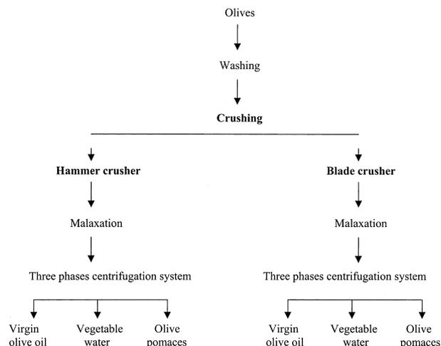
**Fig. 2.** Flux diagram of the processing procedures using hammer and blade crushers.
