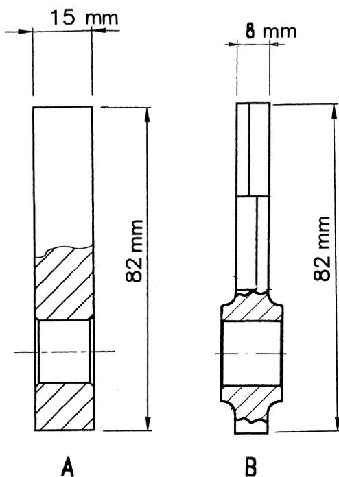
**Fig. 1.** Schematic drawing of the hammer (A) and blade (B) crushing members.
