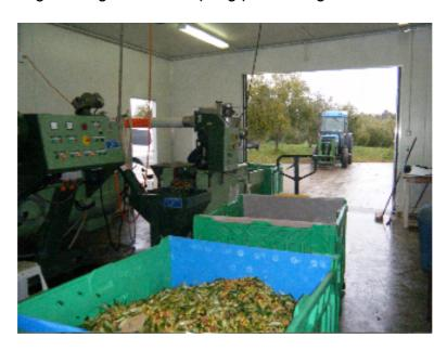
Hammer mill feed auger. This unit is free standing and has a feed hopper, an auger which lifts olives to the hammer mill. Power is from the main press unit control box. This auger has been modified to have a speed controller and reverse, so speed can be altered to suit different olive varieties and degrees of ripeness.
