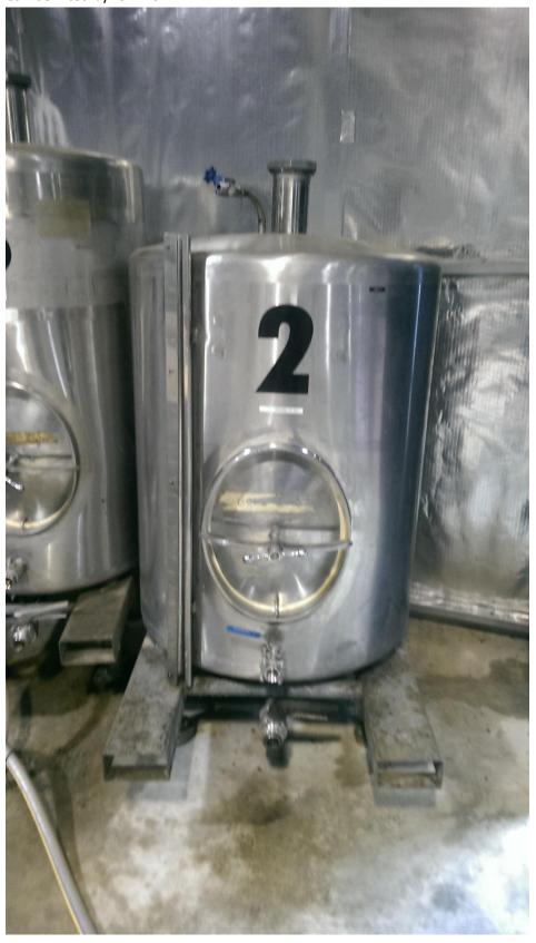
3. 500L\*Lower tap is non standard fitting – needs replacingCan be lifted by forklift
