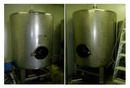
Fittings are 1 and a half inch dairy fittings on valves. Some fittings available to allow effective blending of 5000L between the 2 tanks. Both tanks can be easily moved when empty with a Jiffy truck.
