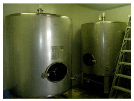
2x 2500L Stainless Steel olive oil tanks. Both custom made for use in olive oil storage from heavy gauge stainless.
