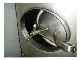
Top 100mm dairy fitting with positive pressure valve. Gas fitting for filling with inert gas. We have used Nitrogen, but Argon could also be used easily.
