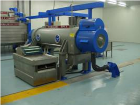
Decanter separating olive oil from paste
